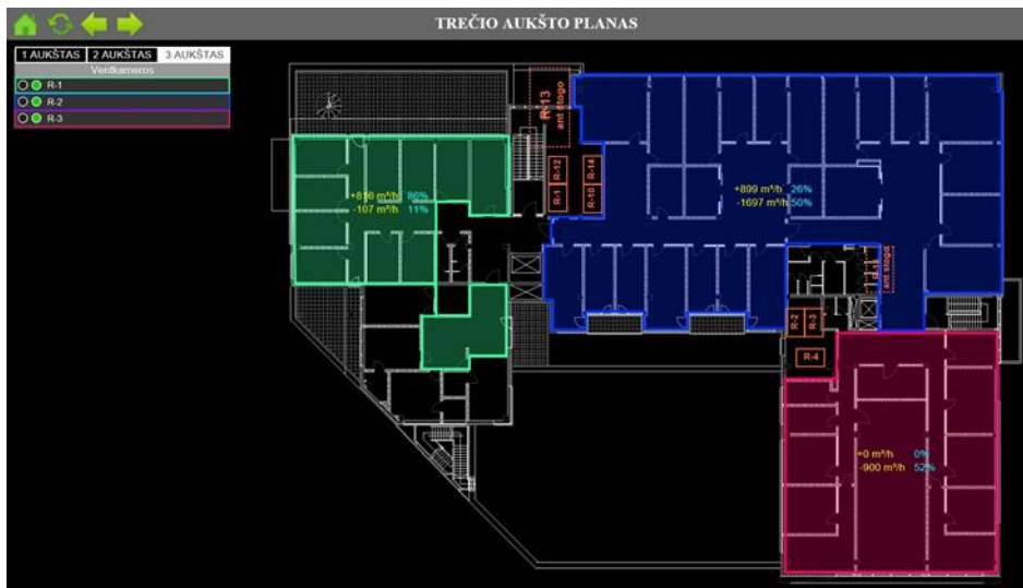
Figure 32. The zoning plan of the ventilation-recuperation system of the third floor of MRI
